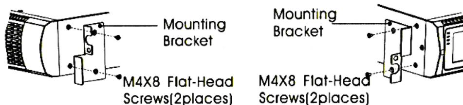
Gambar 4. Pemasangan fixing bracket
